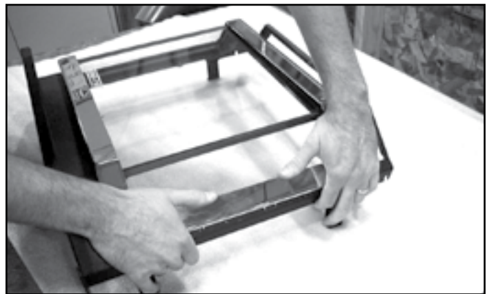
Figure 8.4 - Carefully align the left side of the crown into place, and wrap it across the face of door, finally snapping it into place on the right hand side. Reinsert and tighten the screws previously removed.
