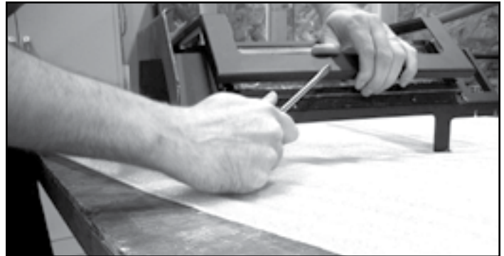
Figure 8.3 - Use a flat-head screwdriver to pry the black crown free on the right side. Remove the crown and discard.
